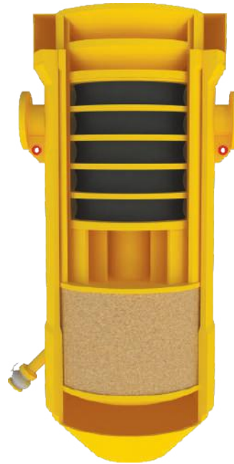
TYPE : B (SHOCK ABSORBER WITH SAND CAN)
