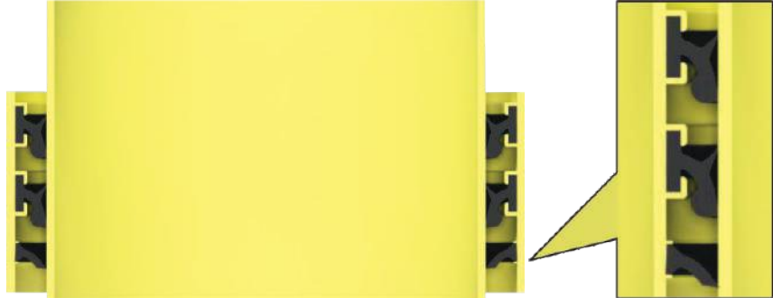
GROUT SEAL WITH MUD VIPER
