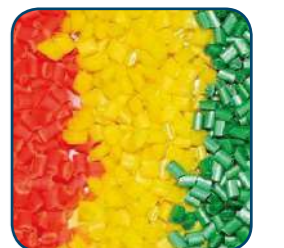
IALA specifications: Pigments integrated into the polyethylene for no painting ever
